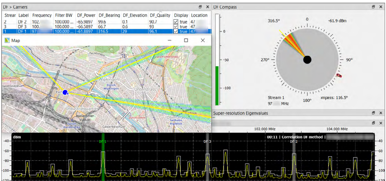
Perform multichannel direction finding and visualize the lines of bearing of all the desired channels
